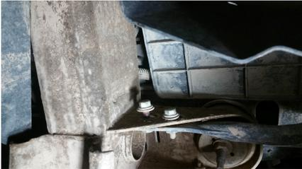
2. On the Driver Side, this bolt must be removed to allow the bracket to slide behind the plastic cover
